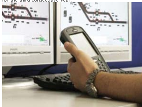
A maintenance technician monitors the status of an in-line baggage system using a wireless device.
